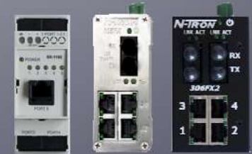
SX-1162 5x port Tx 10SFx 4x Port TX 1x Port FX 306FX2 4x Port TX 2x port FX
